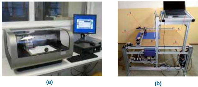
FIGURE 10. (a) Commercial DMP 2831 ink jet printer, (b) Setup of Inkjet printing with simultaneous sintering process on the textile substrate [63].
