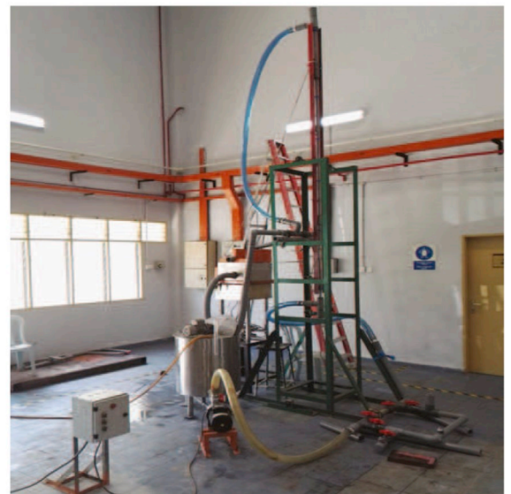
(b) Layout of the flow loop rig simulator.
