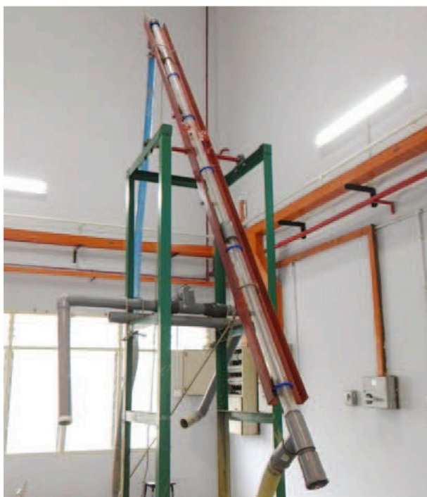
Fig. 7. Annular test section.
