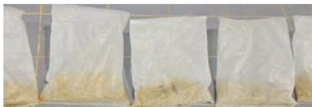
Fig. 3. Simulated drilled cuttings in separated bags.
