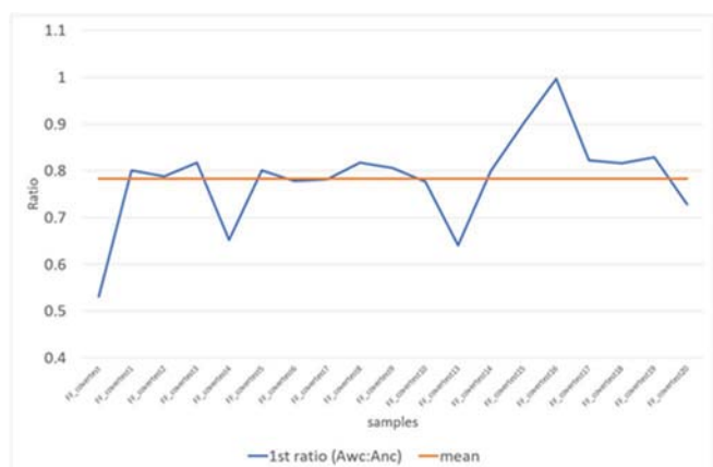
Fig. 10: 1st amplitude ratio of antenna with cover to antenna without cover
