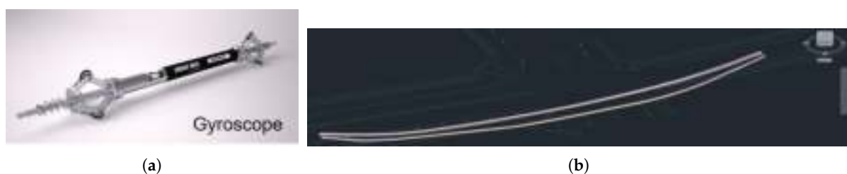
Figure 5. An example of a gyroscope-based pipeline measurement system (a) and the 3D map of the measured pipes (b).
