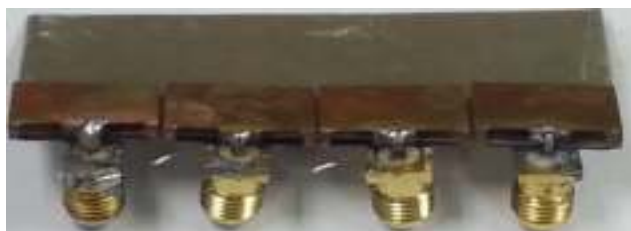
FIGURE 10. Fabricated prototype of 4-Element compact phased PIEA array.
