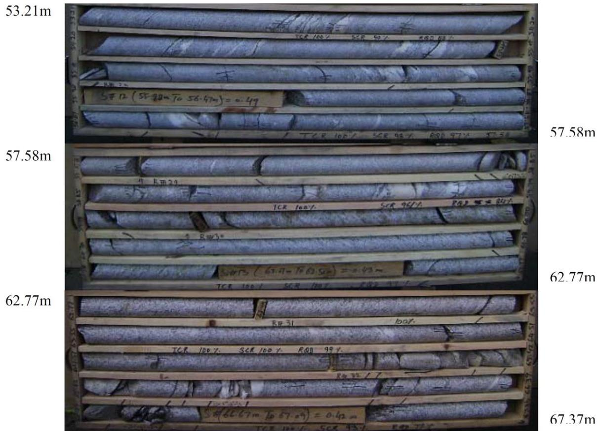
**Figure 8.** Core boxes showing the core recovered from the borehole in the study area.
