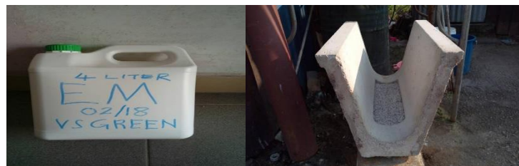
Figure 6. Preparation of eco-composite porous concrete with EM for V-drain.
