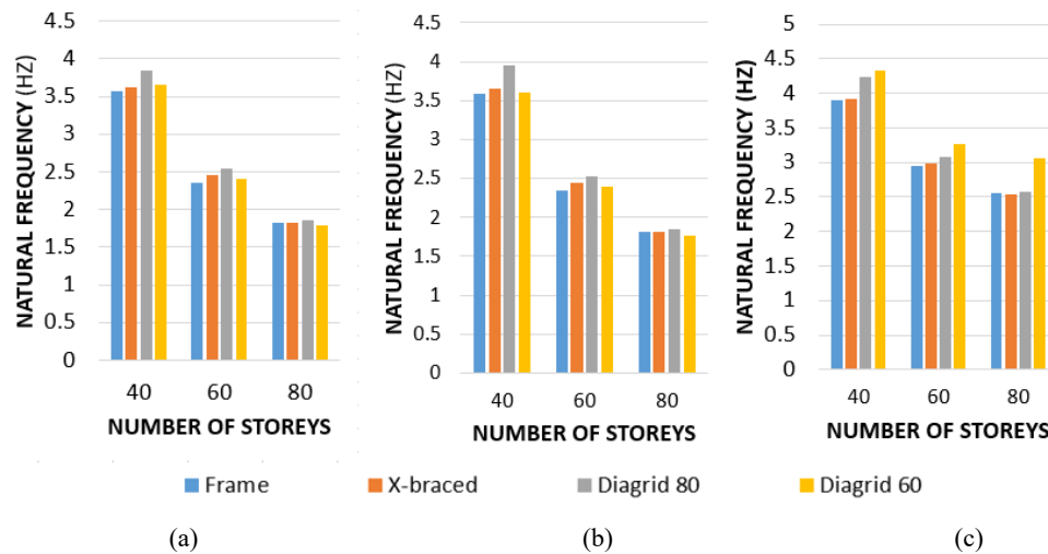
Figure 9. The natural frequency in (a) along wind (b) across wind (c) torsional direction, of building models with different tall building systems.
