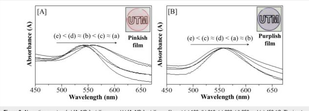
Figure 8: Absorption spectra of a) [AuNPs]<sub>cal</sub>/silica<sub>hex</sub> and b) [AuNPs]<sub>red</sub>/silica<sub>hex</sub> films at (a) 190, (b) 210, (c) 230, (d) 250 and (e) 450 °C. The insets show representative photography images for the as-synthesized films after both heat treatments.
