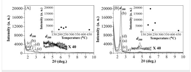
**Figure 4:** XRD patterns in the small-angle region of a) [AuNPs]<sub>cal</sub>/silica<sub>hex</sub> films after calcination and b) [AuNPs]<sub>red</sub>/silica<sub>hex</sub> films after the thermal hydrogen reduction at (a) 190, (b) 210, (c) 230, (d) 250 and (e) 450 °C, where the inset graphs shown the XRD peaks of the maximum intensity of  $d_{100}$  versus temperature.
