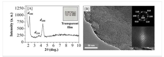
Figure 3: a) XRD diffractogram; the inset is a photograph of the material. b) TEM image; the inset shows the FFT (top) and auto-correlation images (bottom) of [Au<sub>3</sub>Pz<sub>3</sub>]<sub>C10TEG</sub>/silica<sub>hex</sub>.
