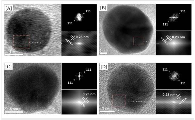
Figure 7: a) TEM images of [AuNPs]<sub>cal</sub>/silica<sub>hex</sub> films at 250 and b) 450 °C as well as c) [AuNPs]<sub>red</sub>/silica<sub>hex</sub> films at 210 and d) 250 °C. The insets show the corresponding FFT patterns (top) and auto-correlation images (bottom).
