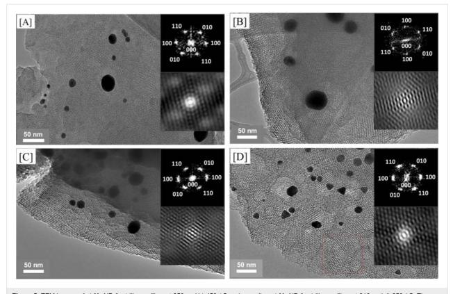
Figure 5: TEM images of a) [AuNPs]<sub>cal</sub>/silica<sub>hex</sub> films at 250 and b) 450 °C and as well as c) [AuNPs]<sub>red</sub>/silica<sub>hex</sub> films at 210 and d) 250 °C. The insets show the corresponding FFT (top) and auto-correlation images (bottom).
