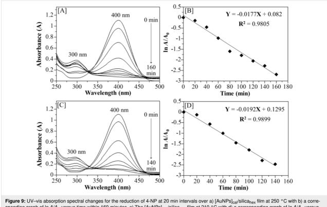
Figure 9: UV-vis absorption spectral changes for the reduction of 4-NP at 20 min intervals over a) [AuNPs]<sub>cal</sub>/silica<sub>hex</sub> film at 250 °C with b) a corresponding graph of  $\ln A/A_0$  versus time within 160 minutes. c) The [AuNPs]<sub>red</sub>/silica<sub>hex</sub> film at 210 °C with d) a corresponding graph of  $\ln A/A_0$  versus time within 140 minutes.
