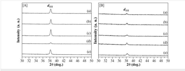
Figure 6: XRD patterns for the wide-angle region of a) [AuNPs]<sub>cal</sub>/silica<sub>hex</sub> and b) [AuNPs]<sub>red</sub>/silica<sub>hex</sub> at (a) 190, (b) 210, (c) 230, (d) 250 and (e) 450 °C.
