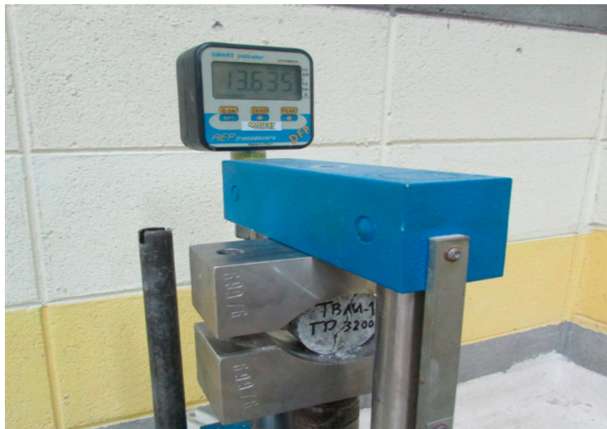
Figure 2. Failure of a sample collected from the tunnel project (tunnel boring machine (TBM) 1, tunnel distance = 3200 m) under Brazilian test.
