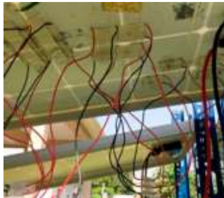
Figure 6. Back view of PV panel with TEG attached.
