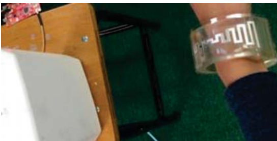
Fig. 4. Fabricated UHF RFID antenna on PDMS material
