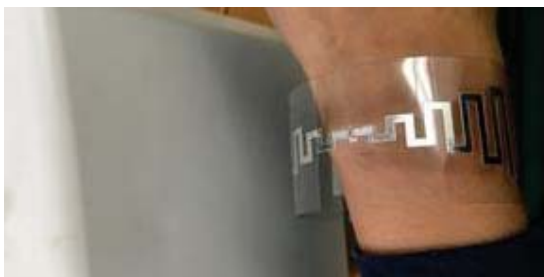
Fig. 3. Fabricated UHF RFID antenna directly on skin
