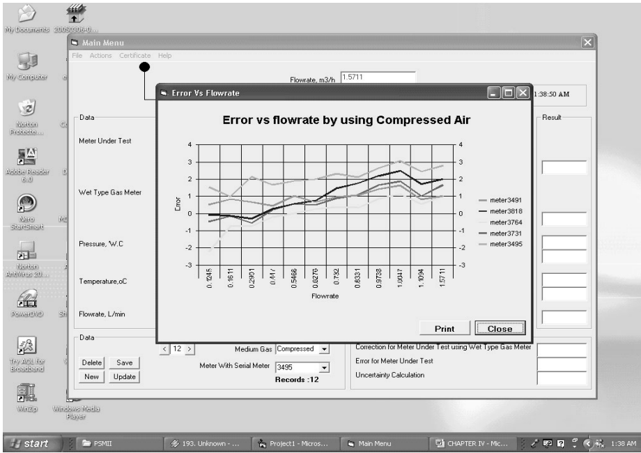
Figure 4.12 Plot of error against flow rate for 5 set of gas meters using compressed air with Visual Basic
