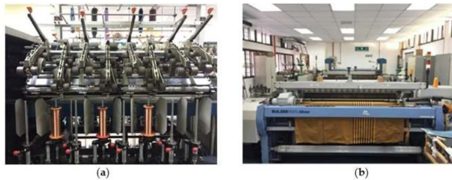
Figure 4. Electro-textile production process: (a) Spindle-spinning process for yarn formation; (b) Weaving process for e-textile formation.
