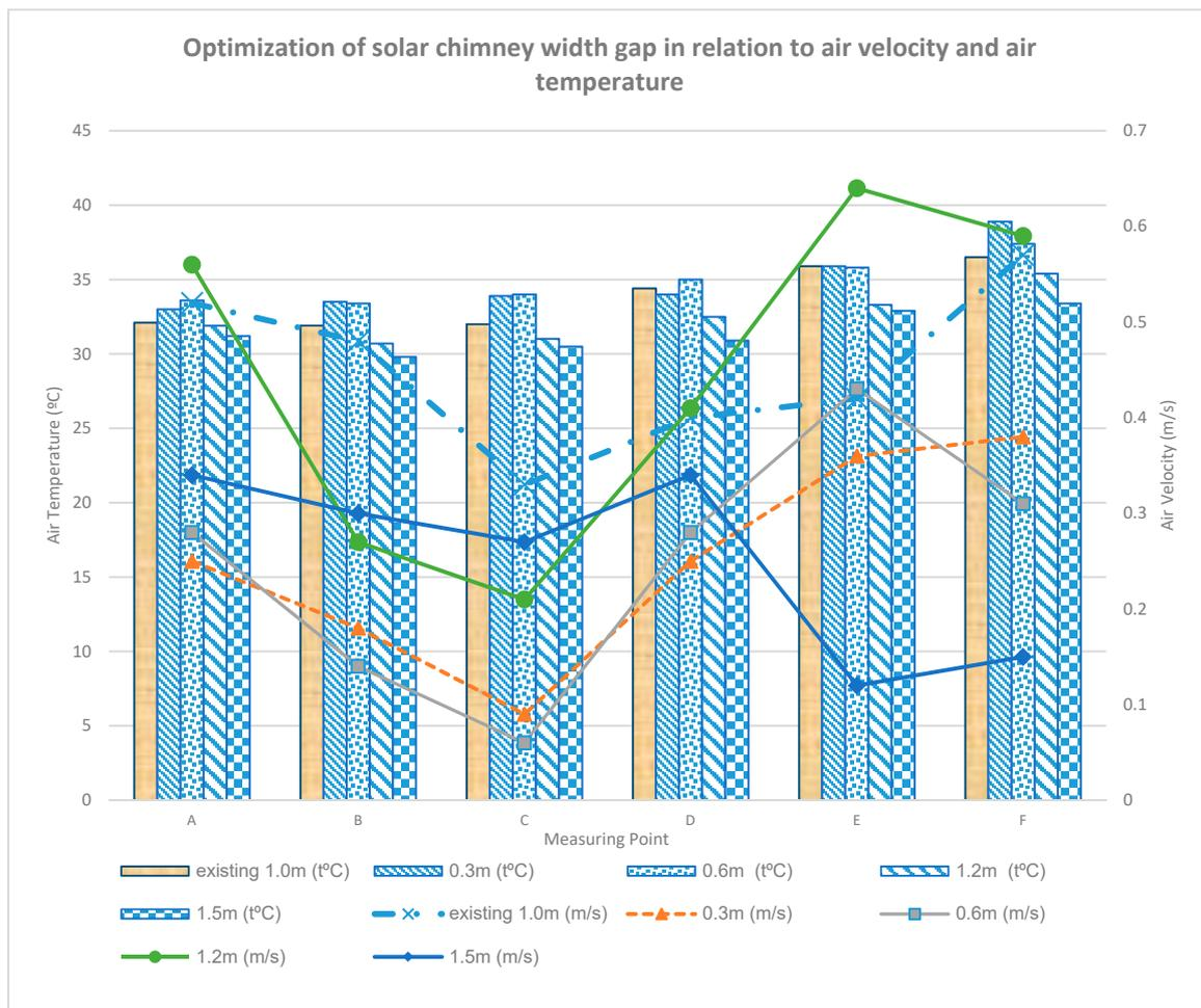
**Figure 13.** Optimization of solar chimney width gap in relation to air velocity and air temperature (6.27).
