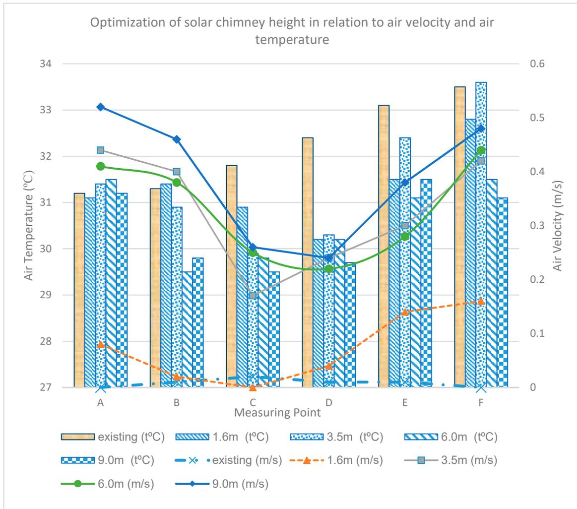
Figure 11. Optimization of solar chimney in relation to air velocity and air temperature (6.25).
