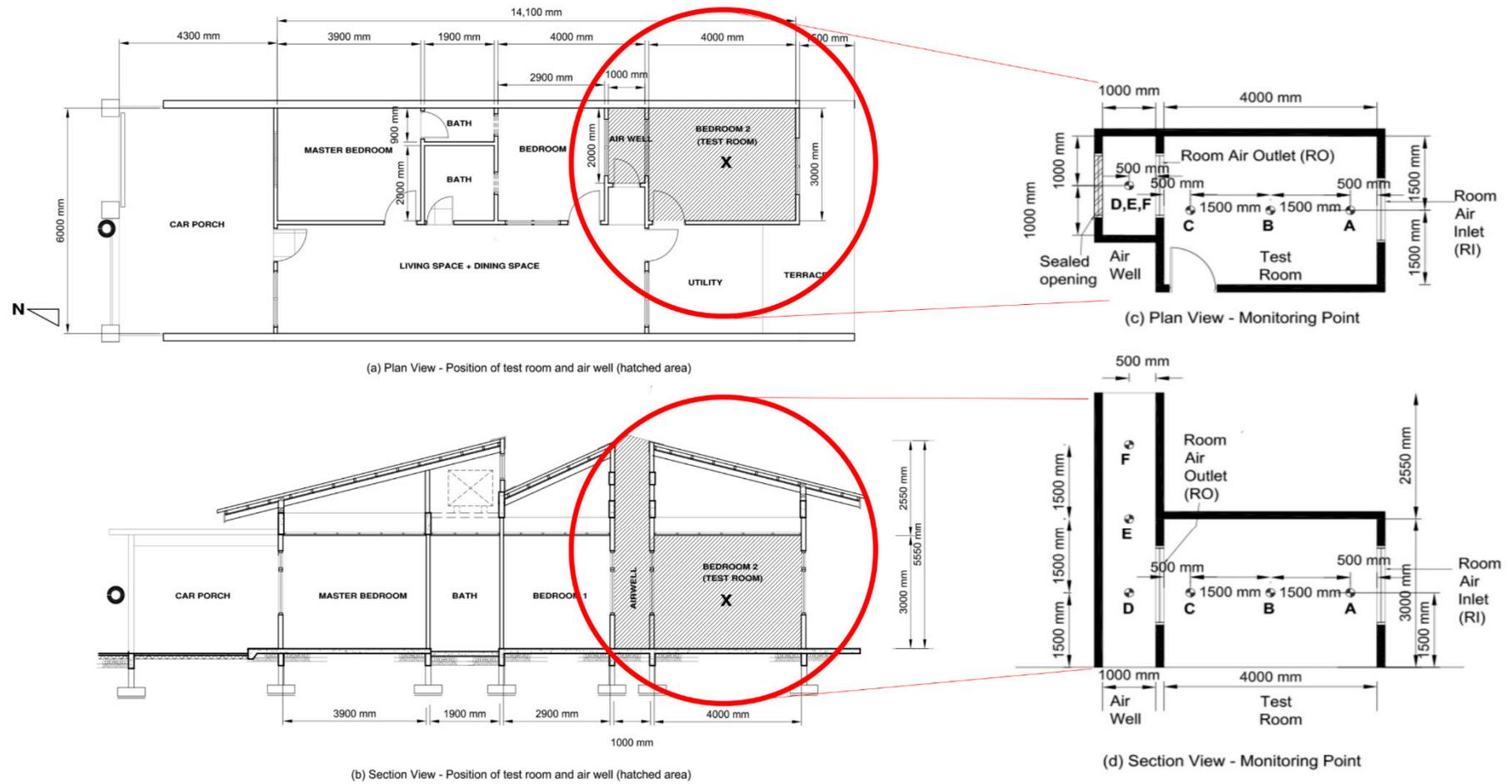
**Figure 10.** Monitoring point for air well/solar chimney model in selected climatic condition: (a) plan view & (b) section view show the position of air well/solar chimney while (c) plan view & (d) section view show the monitoring points for the test room and air well/solar chimney.
