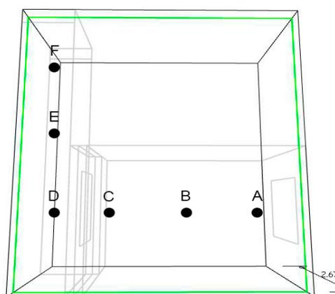
**Figure 8.** Monitoring points of test room and solar chimney in the CFD model (6.23).
