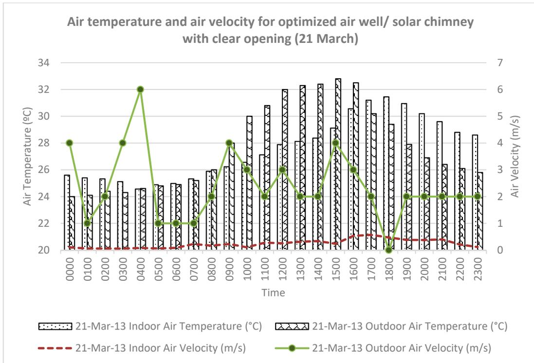
**Figure 18.** Air temperature and air velocity for optimized air well/solar chimney with a clear opening (21 March) (6.32).
