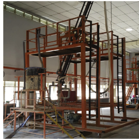
(b) Layout of the flow-loop rig simulator.
