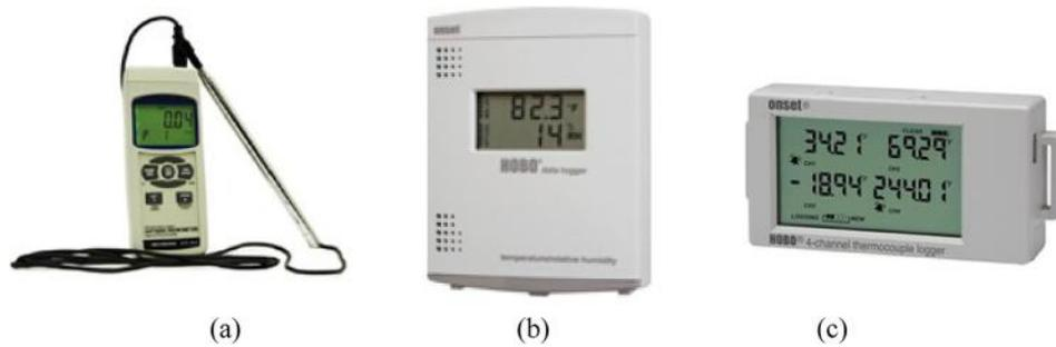
Fig. 3 (a) Hot wire anemometer; (b) temperature & humidity recorder; and (c) HOBO UX120 data logger.
