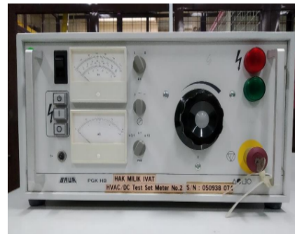
Figure 5. HVAC/DC Test Set Meter
