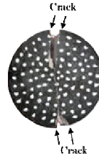
Fig. 12 Specimen after diametrical compression with flat platen 6) .
