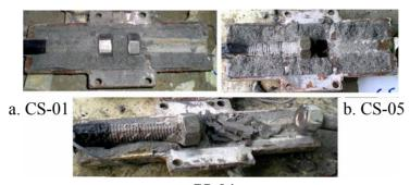
c. CS-04 Figure 13: Failure modes of specimen CS-01, CS-02 and CS-05
