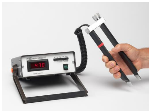
Fig. 2 – Hand grip and pinch digital analyzer from MIE Ltd UK. Picture taken from [31].
