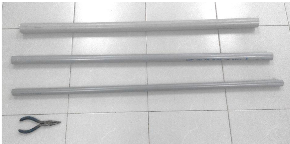
Fig. 2. Pipe of UPVC BS 3505 Class D [16]
