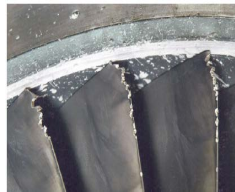
Compressor rotor blades due to foreign object impact, [6]
