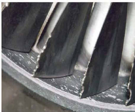
Compressor rotor blades due to foreign object impact, [6]
