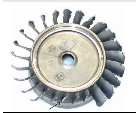
Damaged 4th stage disk, [5]
