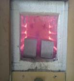
Figure 2 Electric furnace showing concrete specimens
