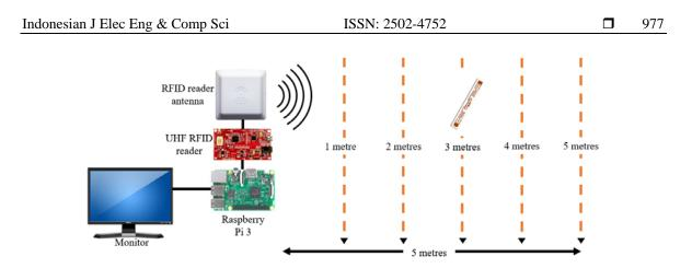
Figure 4. The illustration of setup of measurement
