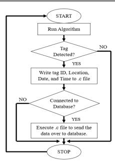
Figure 2. Process flowchart for UHF RFID-Raspberry Pi 3 sensor
