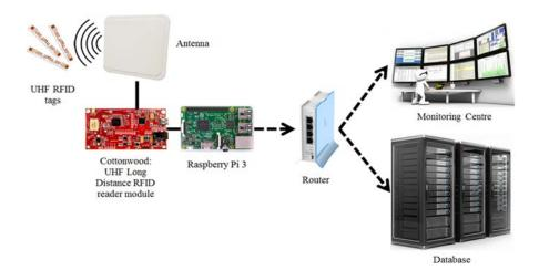
Figure 1. The concept of data transfer of UHF RFID monitoring system
