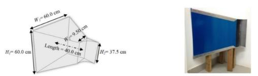
Figure 2. Wind concentrator design's dimension (left: schematic, right: built)
