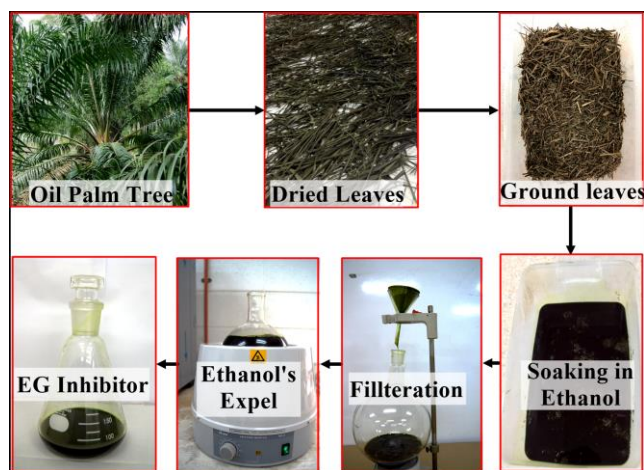
Figure 1 Preparation process of green corrosion inhibitor from Elaeis guineensis leaves
