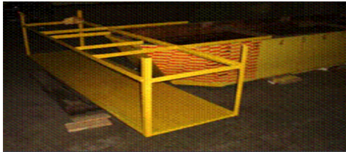
Figure 3: FPSO with submerged plate model
