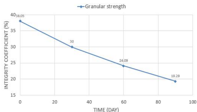
Fig. 8 Strength of aerobic granules cultivated in the SBR.
