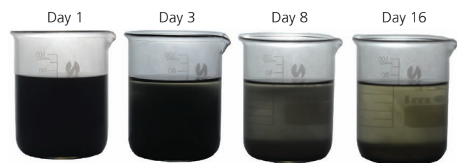
Figure 1. Sedimentation of copper (II) oxide/PKO nanolubricant over a period of time
