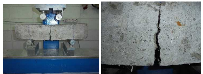
Fig. 9 Cracking failure of Kenaf Fibrous Concrete (KFC)
