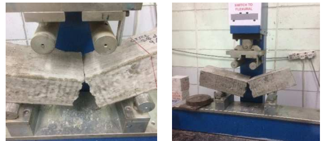
Fig. 8 Cracking failure of Control concrete
