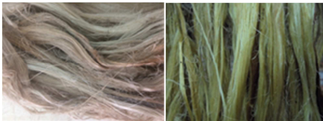
Fig. 1. Kenaf Fiber before and after treatment process
