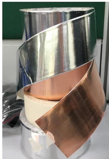
Figure 6. Copper and aluminium tape as radiating element for the antenna tag
