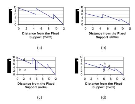
Figure 11. M/EI diagram without the altered section for (a) Trial 1; (b) Trial 2. M/EI diagram when thealtered section is at position 50% for the cantilever beam (c) in Trial 1 (d) in Trial 2.
