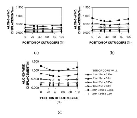
Figure 5. Variation of along-wind displacement in (a) Malaysia (b) New York (c) Hong Kong when the position of the outriggers is altered.
