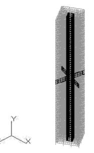
Figure 3.Outrigger and core wall system;
