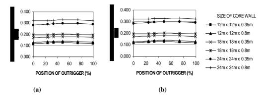
Figure 9. Variation of natural frequency in (a) along-wind direction (b) across-wind direction with different position of outriggers.
