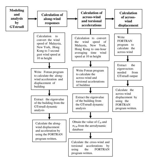
Figure 2. The procedure for the analysis of buildings in this research
