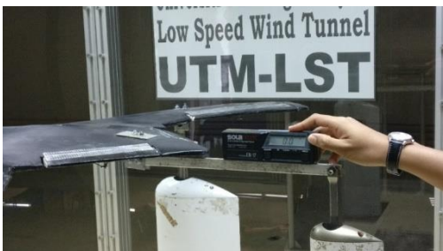
Fig. 6: Model is placed and zero tare method is performed
