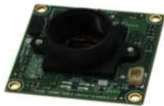
Fig. 2: e-CAM21_CUMI1290_MOD camera models
