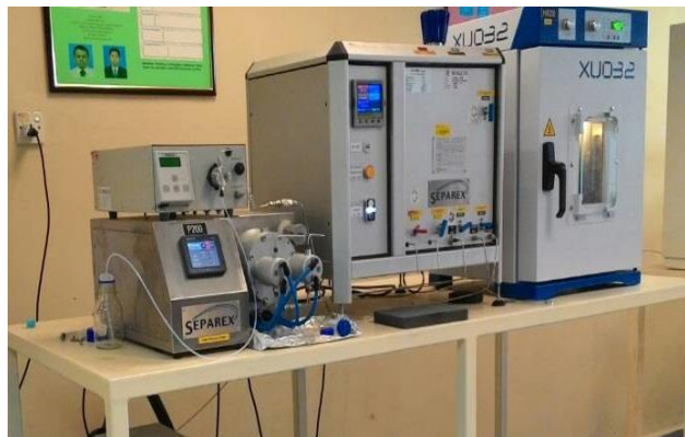
Fig. 2 Supercritical Carbon Dioxide (SC-CO 2 ) Instrument in September 2017 at CLEAR laboratory.
