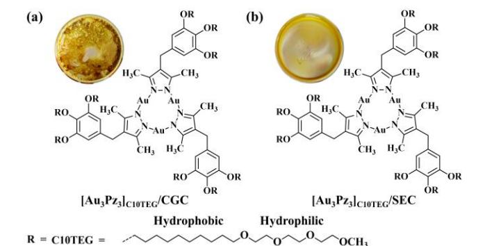
Fig. 2 The chemical structure and visual appearance of [\text{Au}_3\text{Pz}_3]_{\text{C10TEG}} with (a) dark-yellowish color after CGC and (b) pale-yellowish color after recycling SEC.
