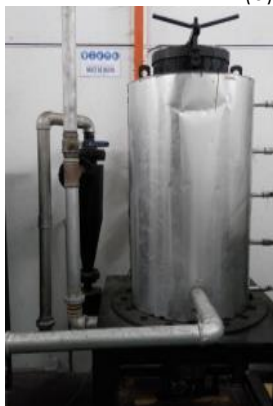
Figure 1 (a) Experiment setup for gasification via downdraft gasifier (b) Downdraft gasifier (c) Schematic of gasification in a downdraft gasifier
