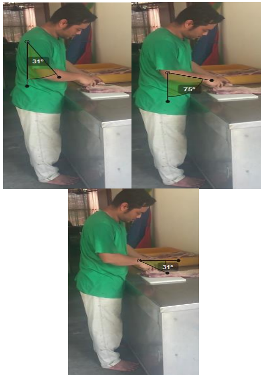
Figure 12 Upper arm, lower arm, and trunk analysis for REBA
