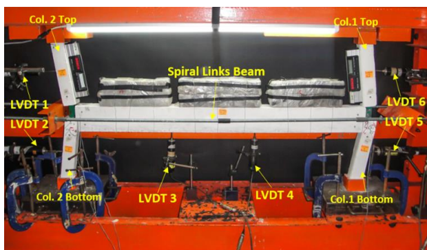
Figure 8 IBSHS model at the end of cyclic loading test (collapse)
