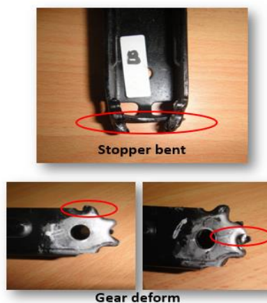
Figure 1. Actual defective sample collected from market
