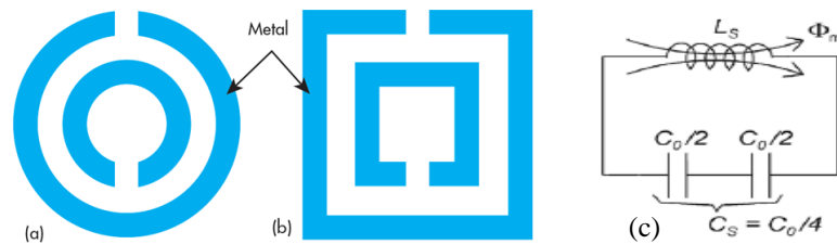
Figure 1. Topologies of (a) Circular SRR (b) Square SRR (c) Their equivalent-circuit model [15]
