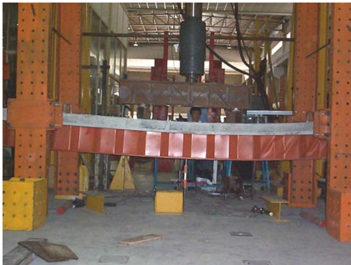
Figure 11 : Failure of TWP-composite specimen due to web buckling near support
