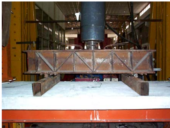
Figure 5 : Free roller used at loading point and rollers for line load spreaders
