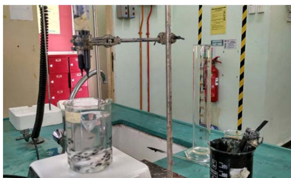
Figure 1: Image of immobilised cell-alginate-graphite preparation.
