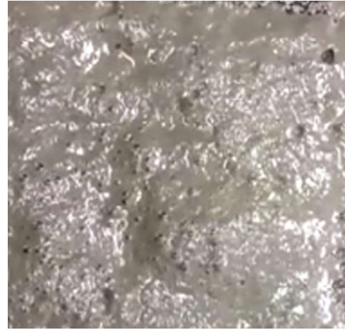
Fig. 1 — Bubbles found when SP and PYE were added to the mix
