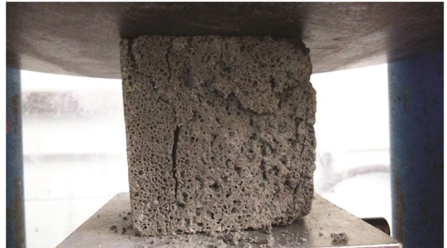
Fig. 2 — Typical fracture after compressive test
