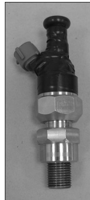
Figure 5: EFIC Flowchart Figure 6: The prototype gasoline direct-injector
