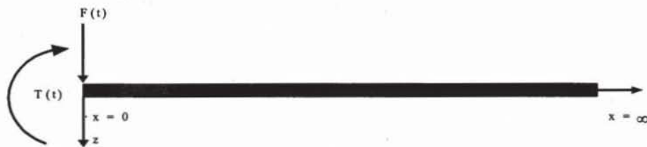
Figure 1 A semi-infinite beam subjected to simultaneous action of bending force and moment excitations.
