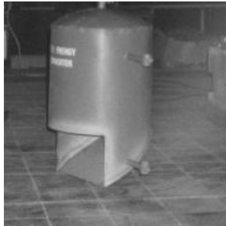
Figure 4: Photo of the Model Test shows the Slope of the Reflector
