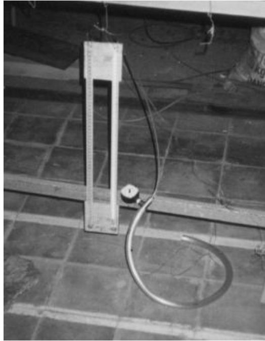
Figure 5: 'U' pipe equipment shows the manometer for calibration work
