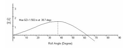
Figure 4: Hydrostatic roll stability of the struck ship
