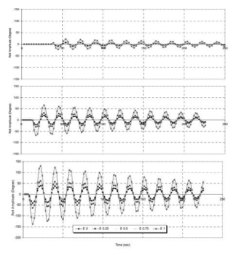
Figure 8: Rolling of struck ship hit 90 deg. at speeds of 1, 3 & 6 knots (top to bottom)
