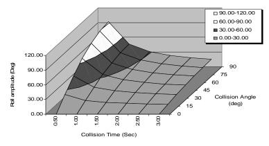
Figure 5: Maximum roll amplitude against collision time and collision angle
