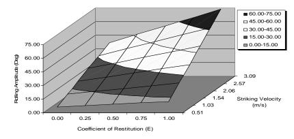
Figure 6: Maximum roll amplitude against coefficient of restitution & striking velocity
