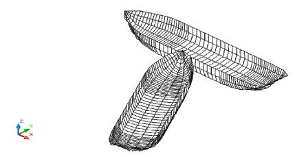
Figure 3: A three dimensional mesh of two ships under collision
