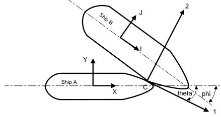
Figure 1: Co-ordinate system of a ship-ship collision
