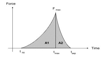
Figure 2: Collision force is an exponential function over the contact period
