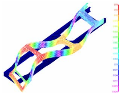
Mode 4: 51.33 Hz Global: 3 nodal points lateral bending
